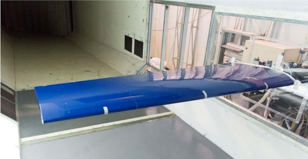
Figure 2: Detail of wind tunnel model installation.
