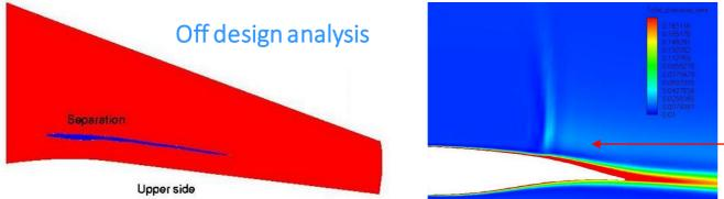
Shock development in off design condition and interaction with boundary layer
