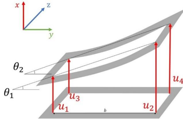
Following equation was used for calculate each angle of a single quadrant into the collimator frame, expressed as a function of the **displacements** along all directions:
