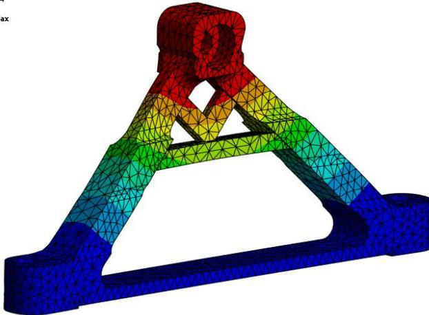
Starting with a natural frequency of **122.7 Hz** to **149 Hz** (+ 15%) with an preliminary increase in mass of 10 g each bipod (+ 16%) reduced with a morphing optimization of 16 g for bipod (**- 18%**).
