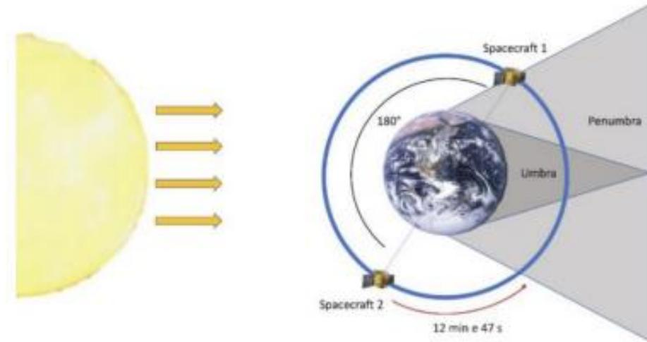
The two small satellites travel at 180° phase difference along the orbit, this configuration ensures **continuous monitoring** of the Sun. This configuration allows to have always at least one satellite of the constellation in daylight for observing the Sun.
