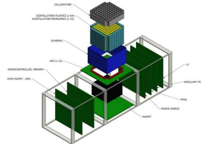
Starting with a simplified concept, based on a first survey on the sensors, with the acceptance of the proposal by the Italian Space Agency, a detailed mechanical design was developed:
