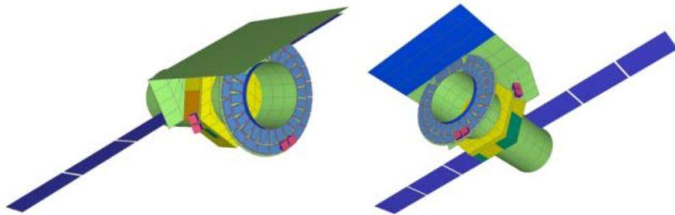
One **detailed module** at each simulation and simplify the remaining 39 modules in terms of mesh refinement (the number of nodes of each component was reduced), with a consequent simplified features for thermal links and dissipations
