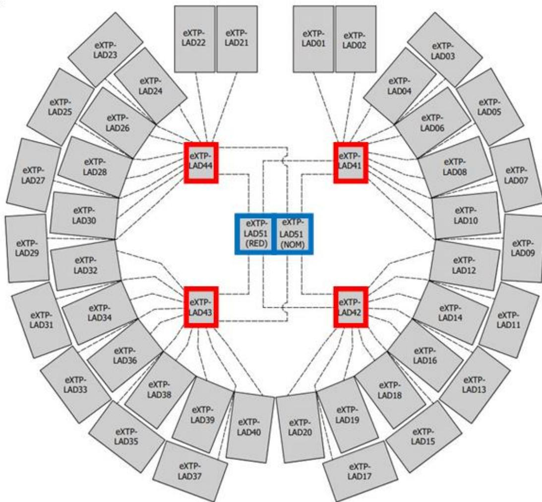
The **Large Area Detector (LAD)** is designed to be the most sensitive spectral-timing instrument for bright Galactic and extra galactic sources to date, an innovative and highly efficient technology and design allow to deploy in space an effective area as **large** as  $3.2 \text{ m}^2$  – class with a modular configuration.
