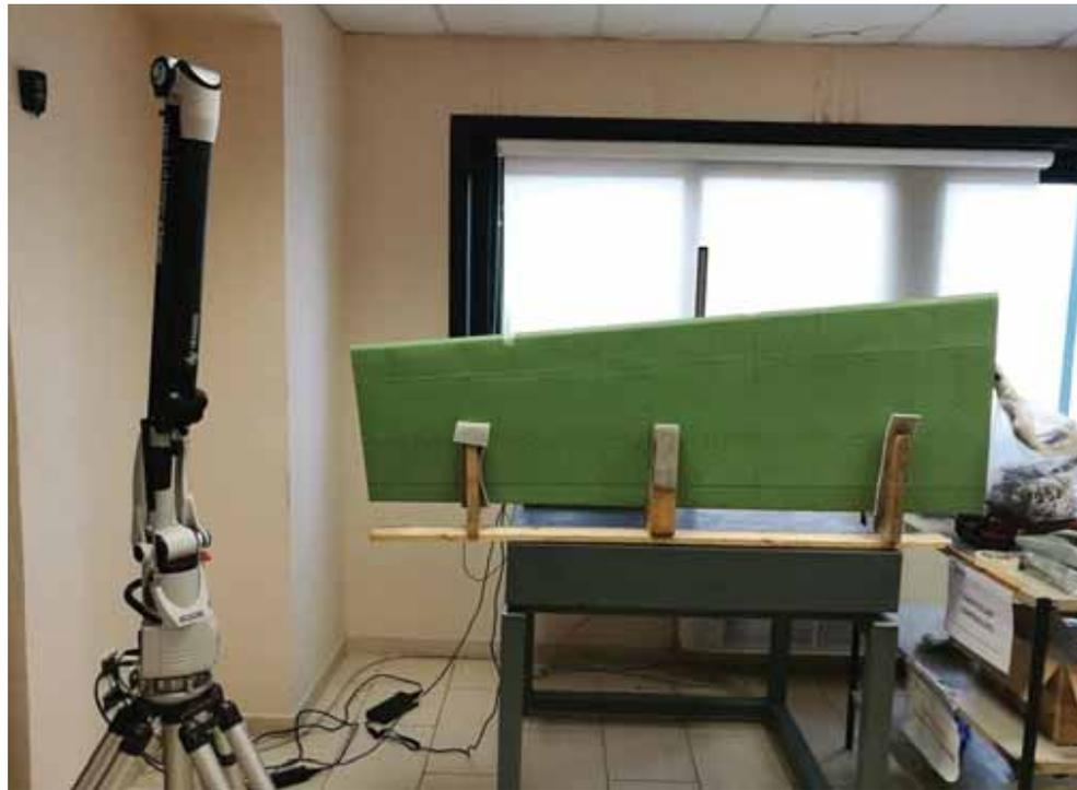
The model geometry has been also reconstructed through a **HEXAGON metrology electronic arm**
