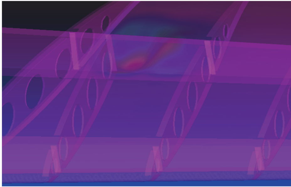
Figure 60 Buckling Zone corresponding to a rib's missing tail
