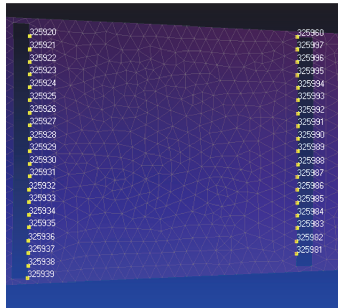
Figure 54 Points used to evaluate plate's average displacement
