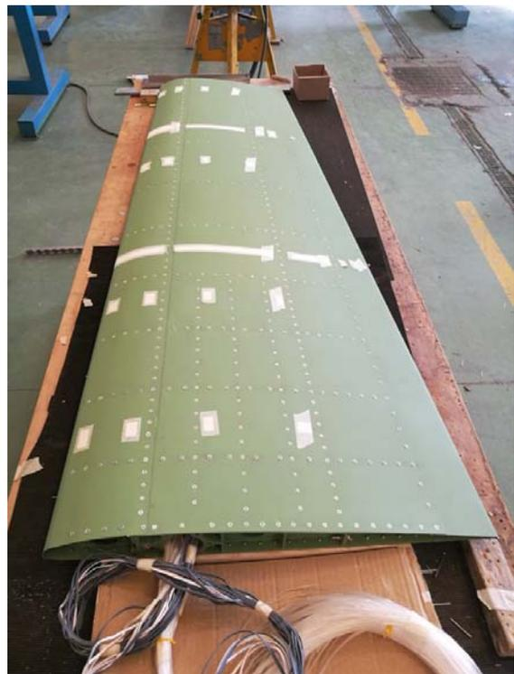
**Figure 68 – Leading edge skin final riveting**
