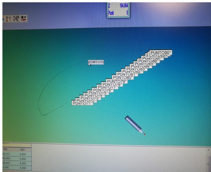
Figure 71 – Wing model section reconstruction with HEXAGON metrology harm.
