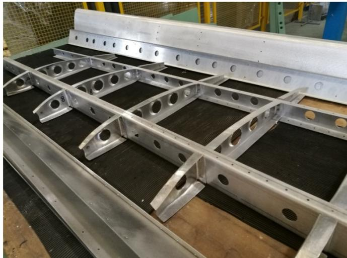
Figure 2: Detail of spars and ribs.
