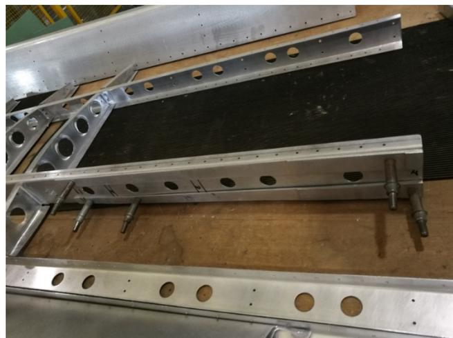
Figure 3: Detail of front spar thickening.
