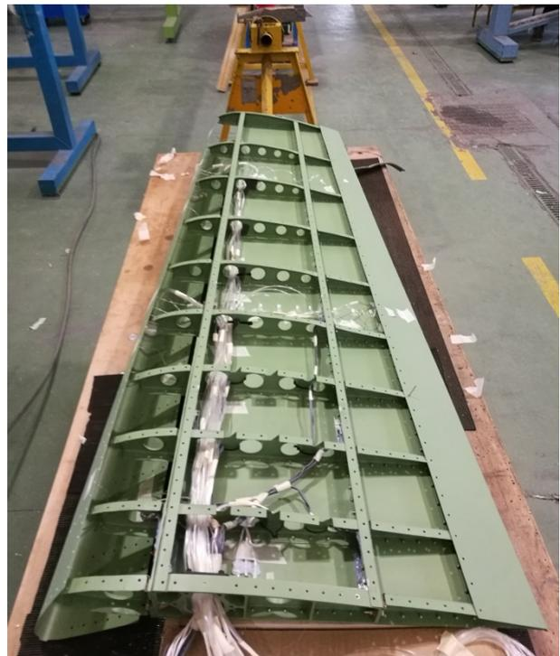
Figure 56 – Leading edge skin wiring
