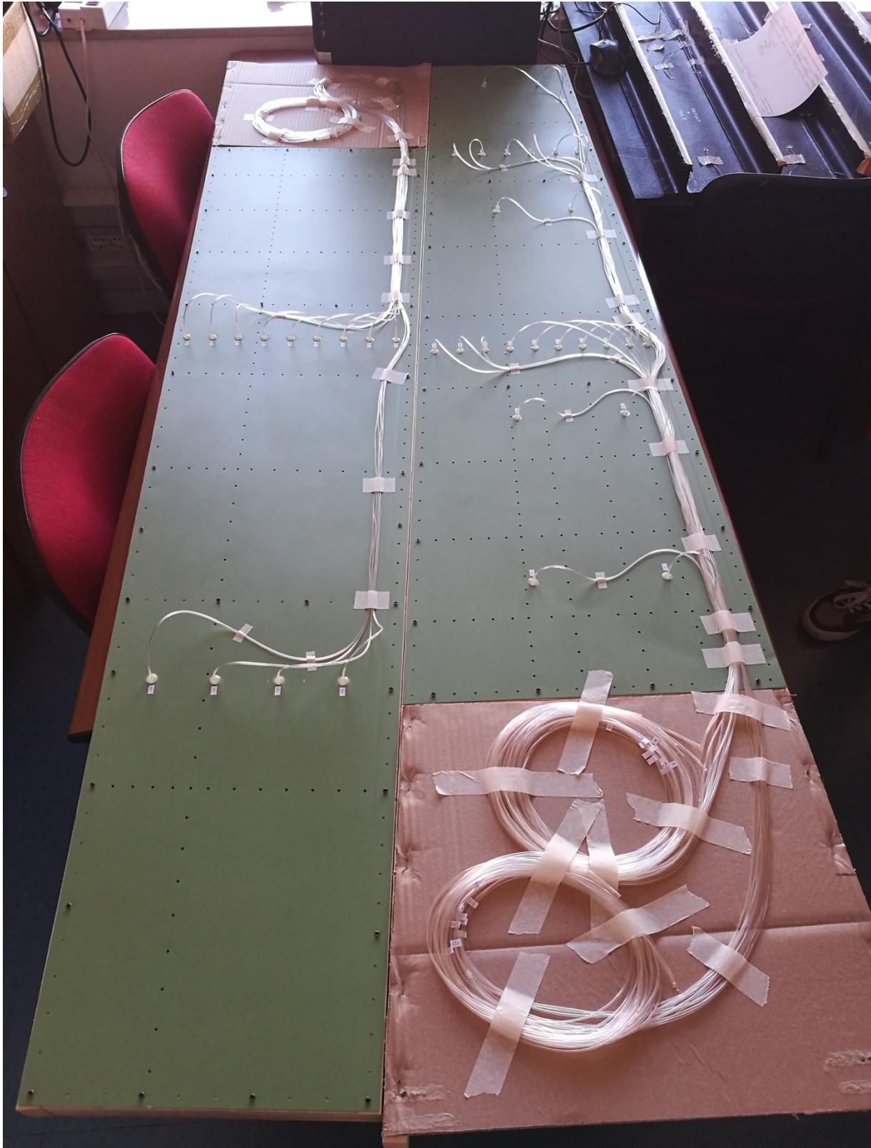
Figure 25 –Pressure taps installed on the upper and lower skin
