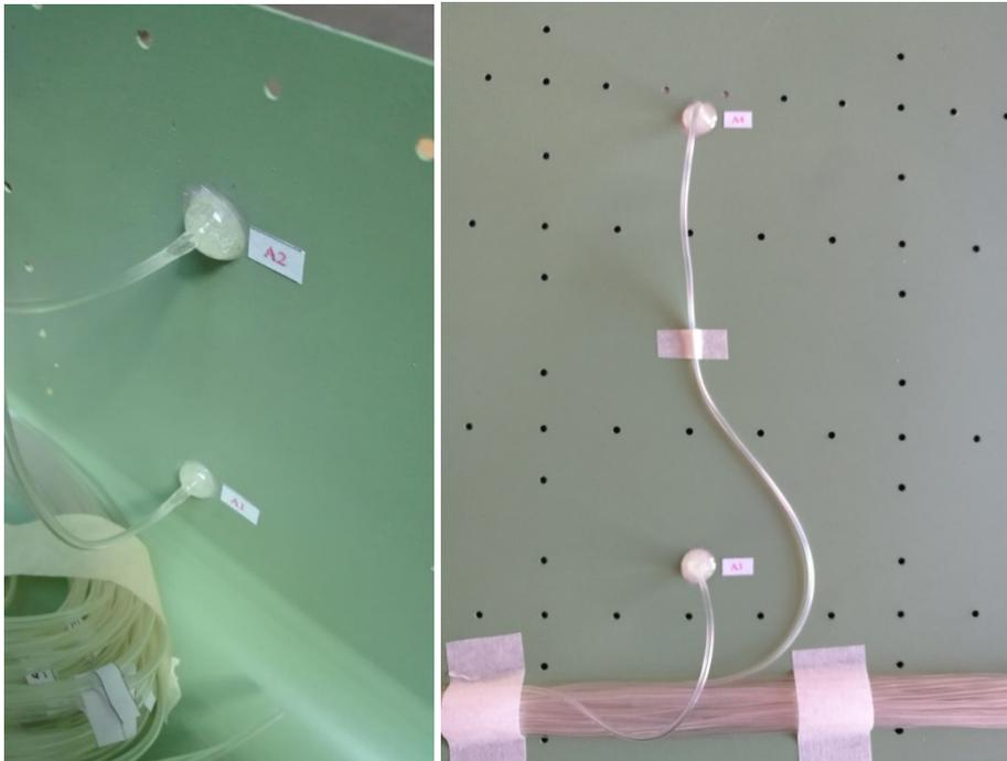
Figure 19 – Section A,  $y=160\text{mm}$ , pressure taps installed
