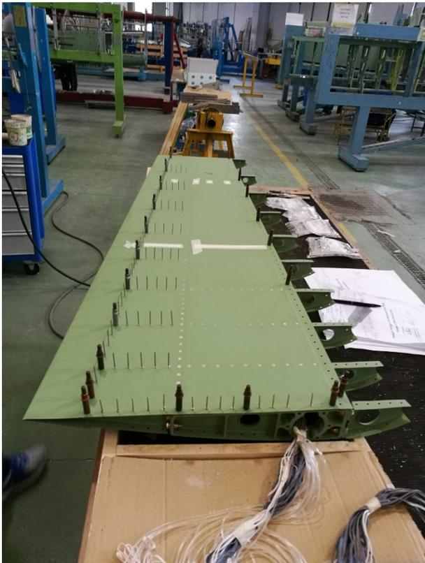
Figure 51 – Trailing edge riveting
