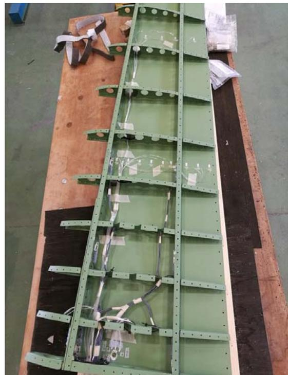
Figure 48 – Lower skin final configuration (detail of cables)
