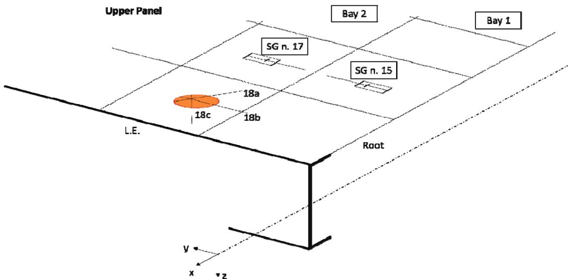
Figure 39 – Position of SGs (white elements) and rosette (orange element) installed on the upper skin.
