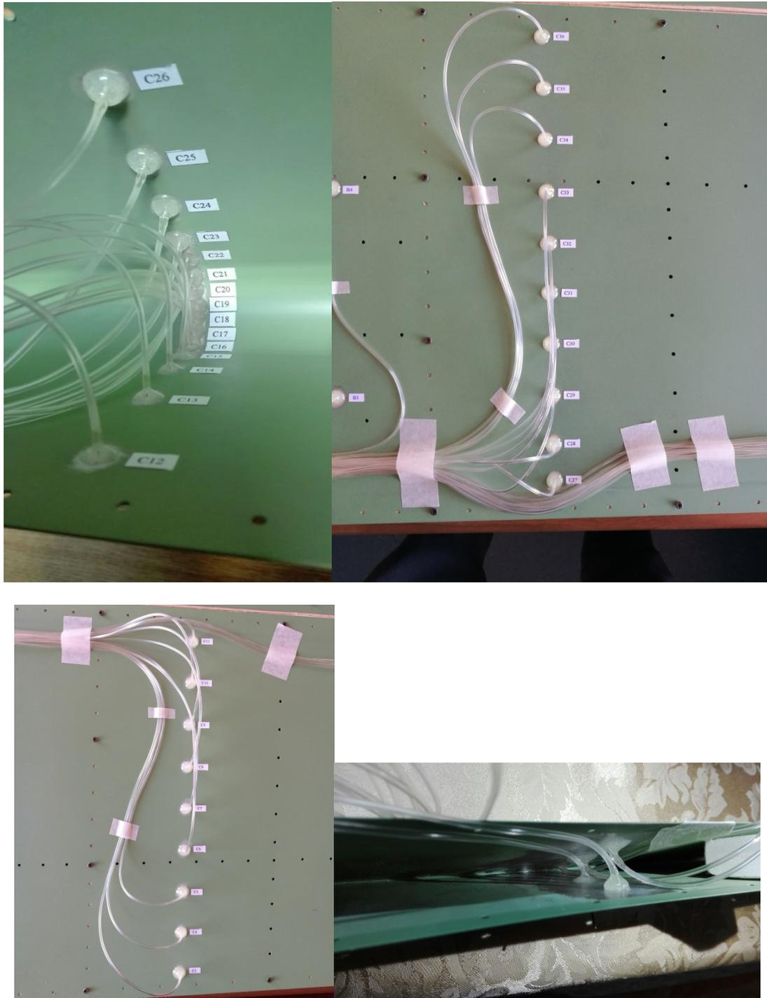
Figure 21 – Section C, y=600mm, pressure taps installed
