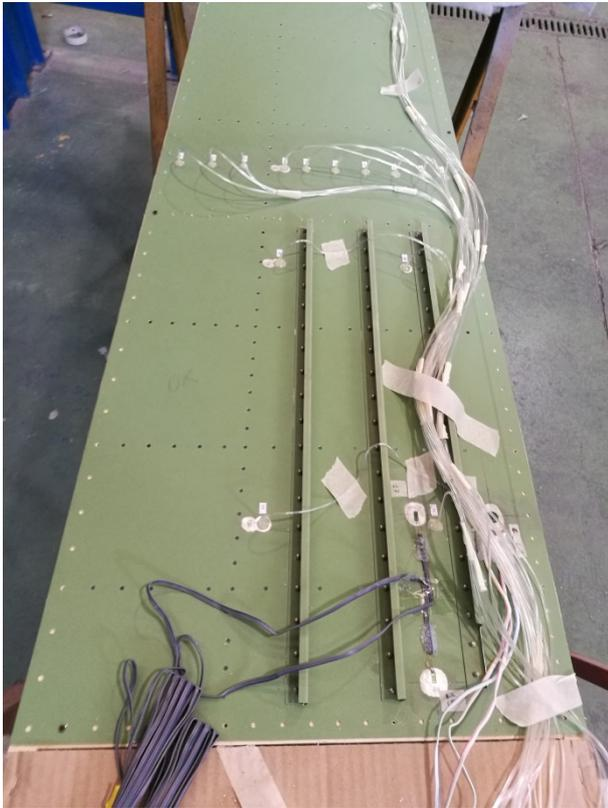
**Figure 57 – Upper skin stringers positioning, wiring**
