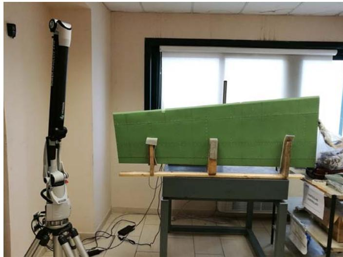
Figure 70 – Wing model in the metrology room, HEXAGON metrology harm
