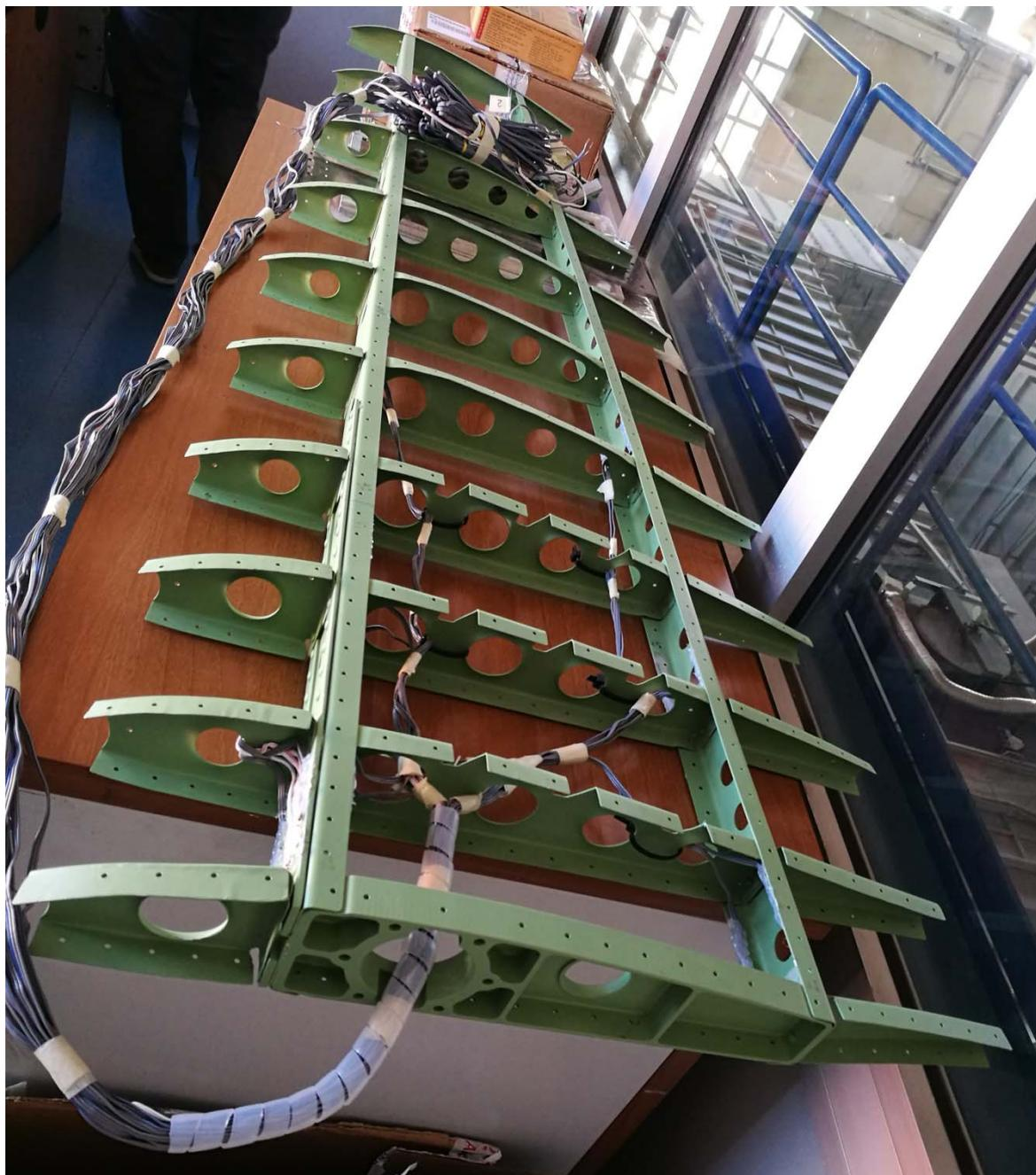
Figure 41 – Strain gauges installed on the internal structure.
