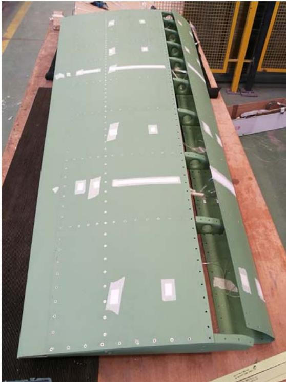
**Figure 65 – Leading edge skin last part to be riveted**
