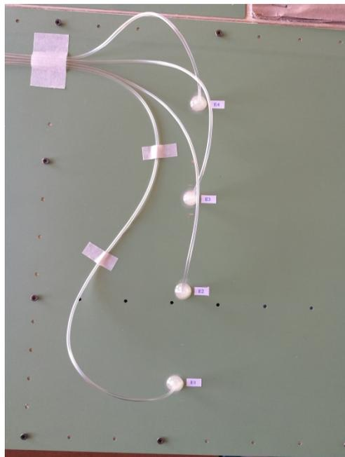
Figure 23 – Section E, y=1200mm, pressure taps installed
