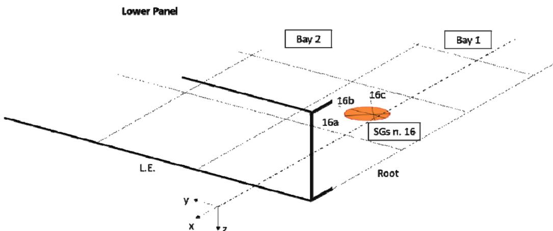
Figure 40 – Position of rosette n.16 (orange element) installed on the lower skin.
