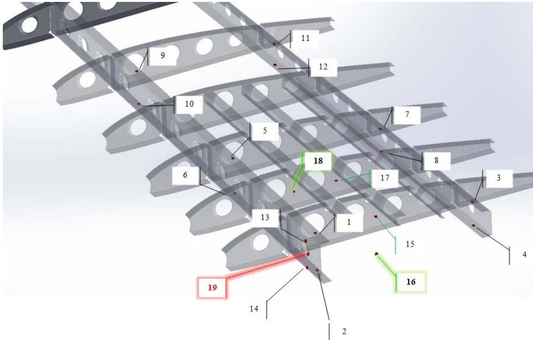
Figure 26 – Strain gauges installation, 15 on the spars, 4 on the skin.
