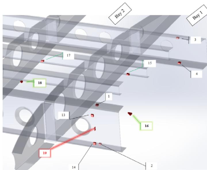
Figure 28 – Strain gauges installation, 15 on the spars, 4 on the skin, bays 1 and 2.
