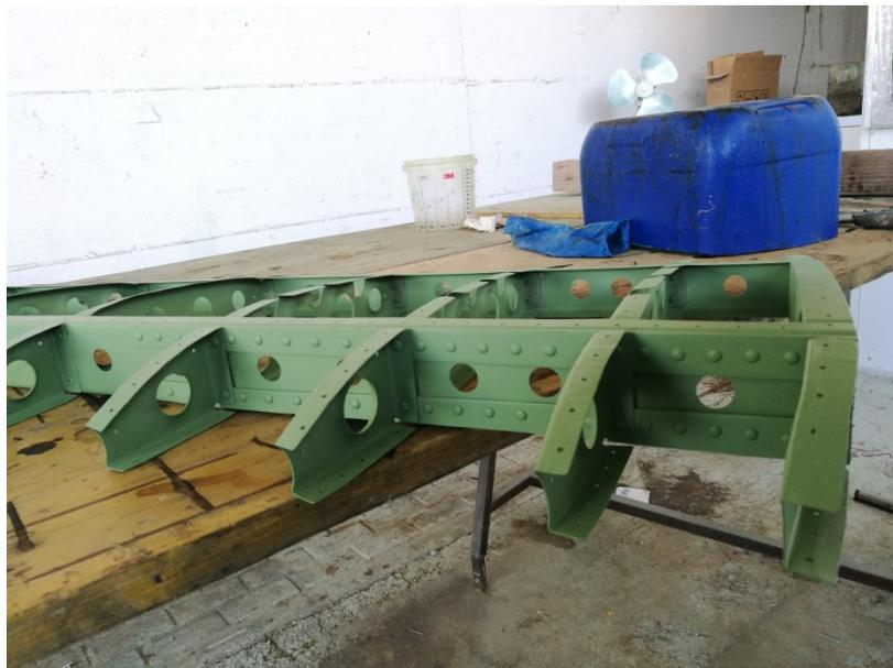
Figure 9: – Front spar thickening nailing.
