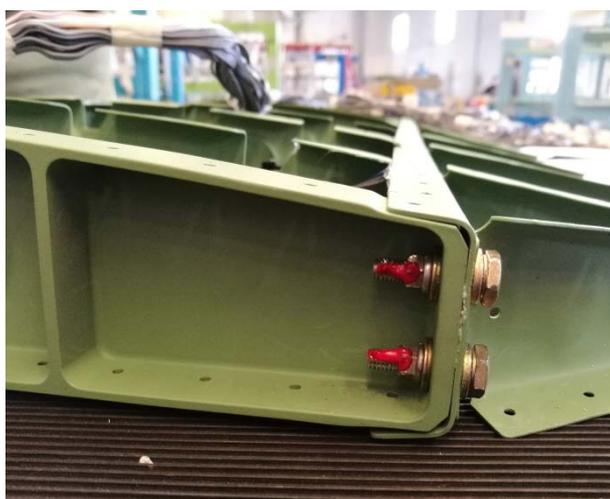
Figure 12 – Rear spar nuts
