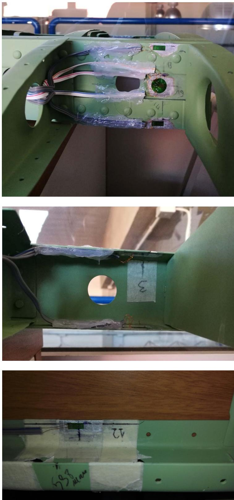
Figure 42 – Details of strain gauges installed on the internal structure.
