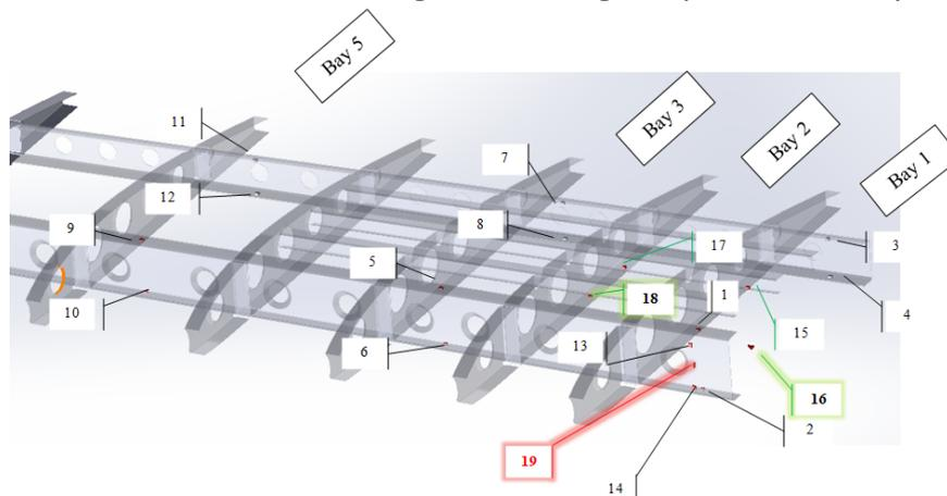
Figure 27 – Strain gauges installation, 15 on the spars, 4 on the skin, bays.
