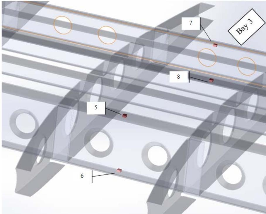
Figure 29 – Strain gauges installation, 15 on the spars, 4 on the skin, bay 3.
