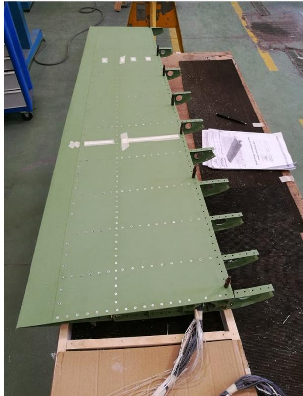
Figure 52 – Trailing edge riveting and final configuration
