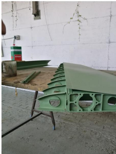
Figure 5: Primer treatment on the entire structure.
