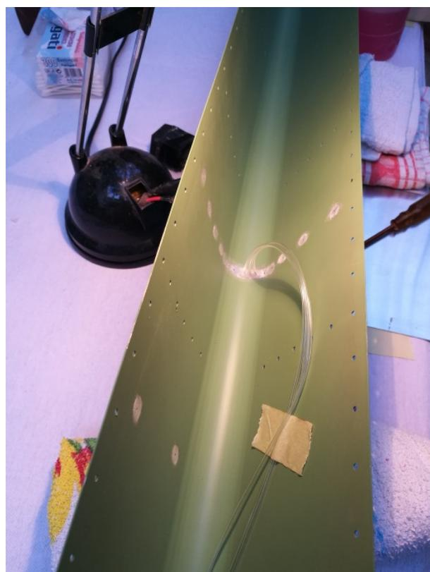
Figure 17 – Leading Edge pressure taps installation
