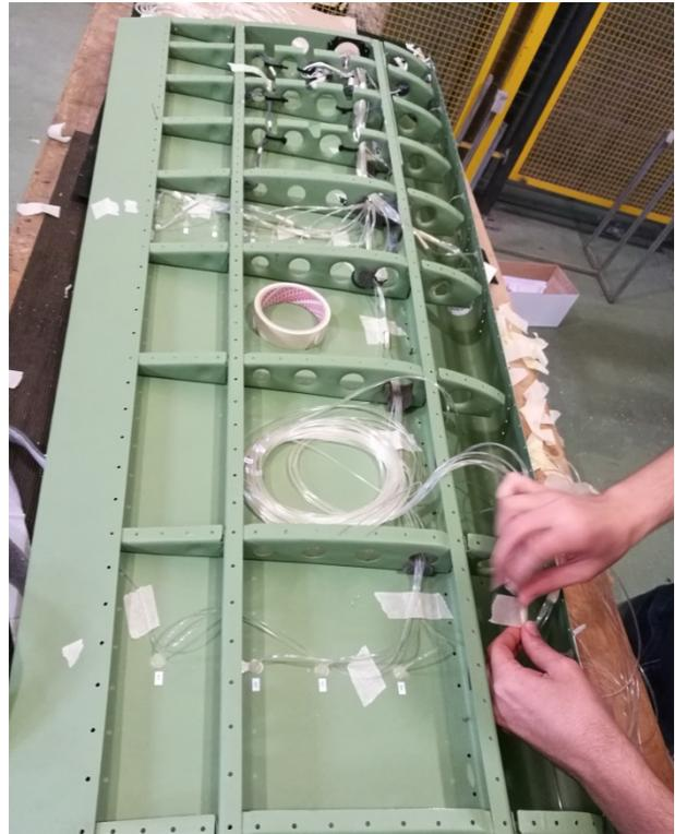
Figure 54 – Leading edge skin wiring
