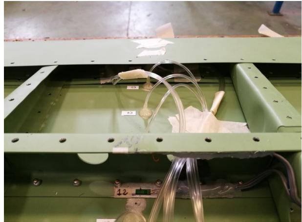
**Figure 50 – Lower skin wiring, detail of SG 12 and pressure taps**
