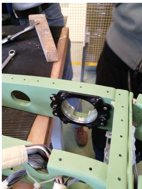
Figure 11 – Rib 1 internal plate
