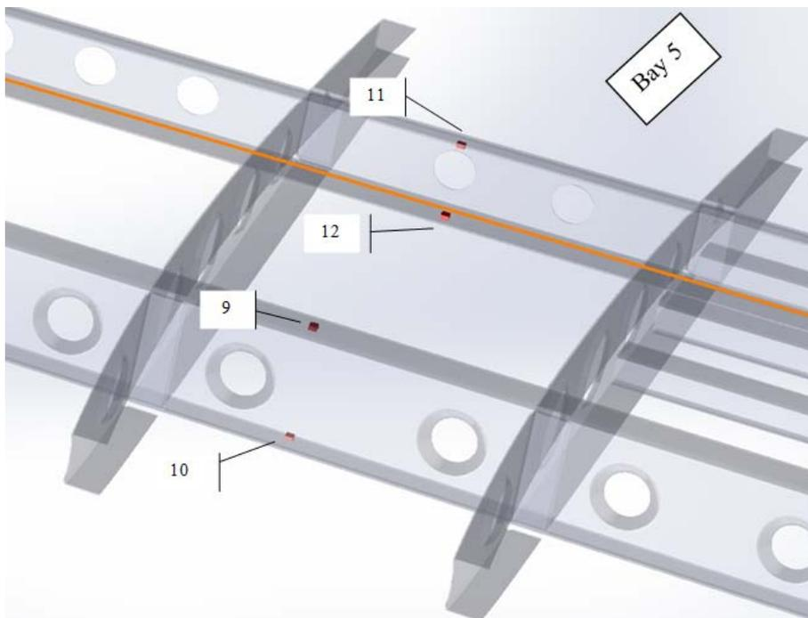
Figure 30 – Strain gauges installation, 15 on the spars, 4 on the skin, bay 5.
