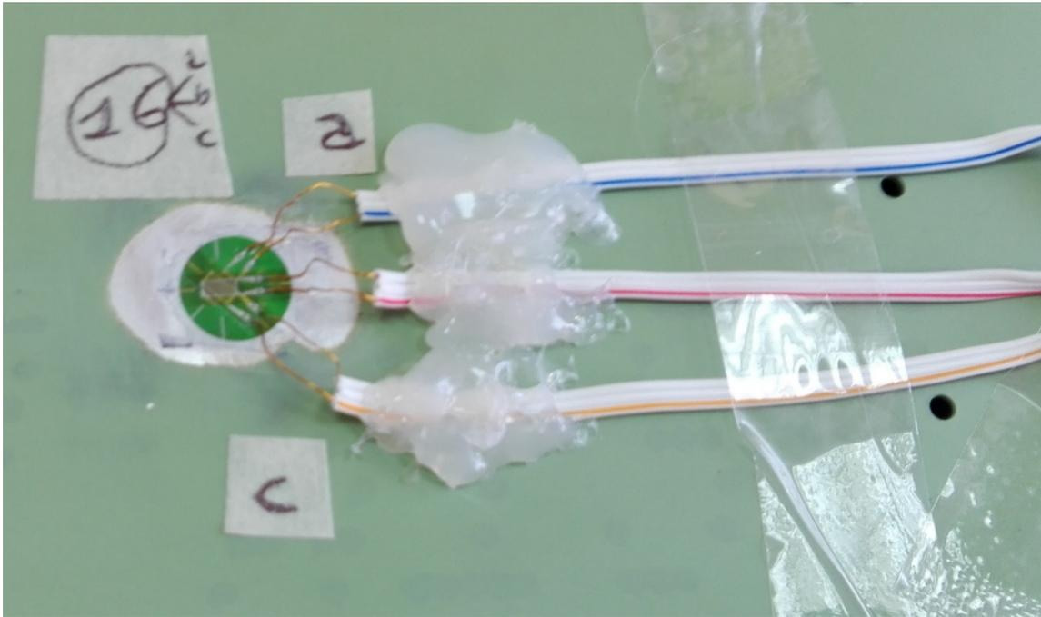
Figure 36 – Hand pressing for the adhesive bonding of the SG on the surface
