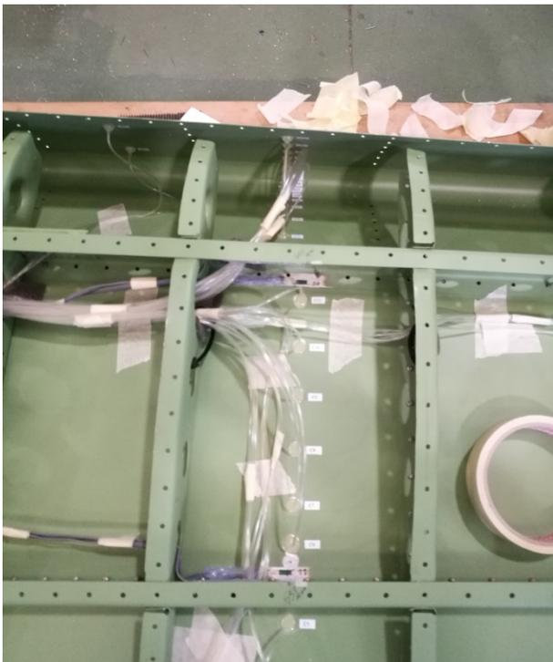
Figure 55 – Leading edge wiring details of cables
