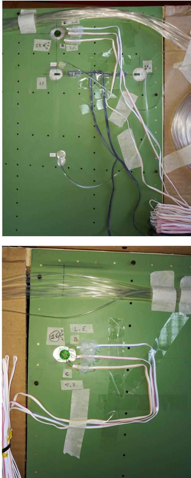
Figure 43 – Details of strain gauges installed on the upper (up) and lower skin.
