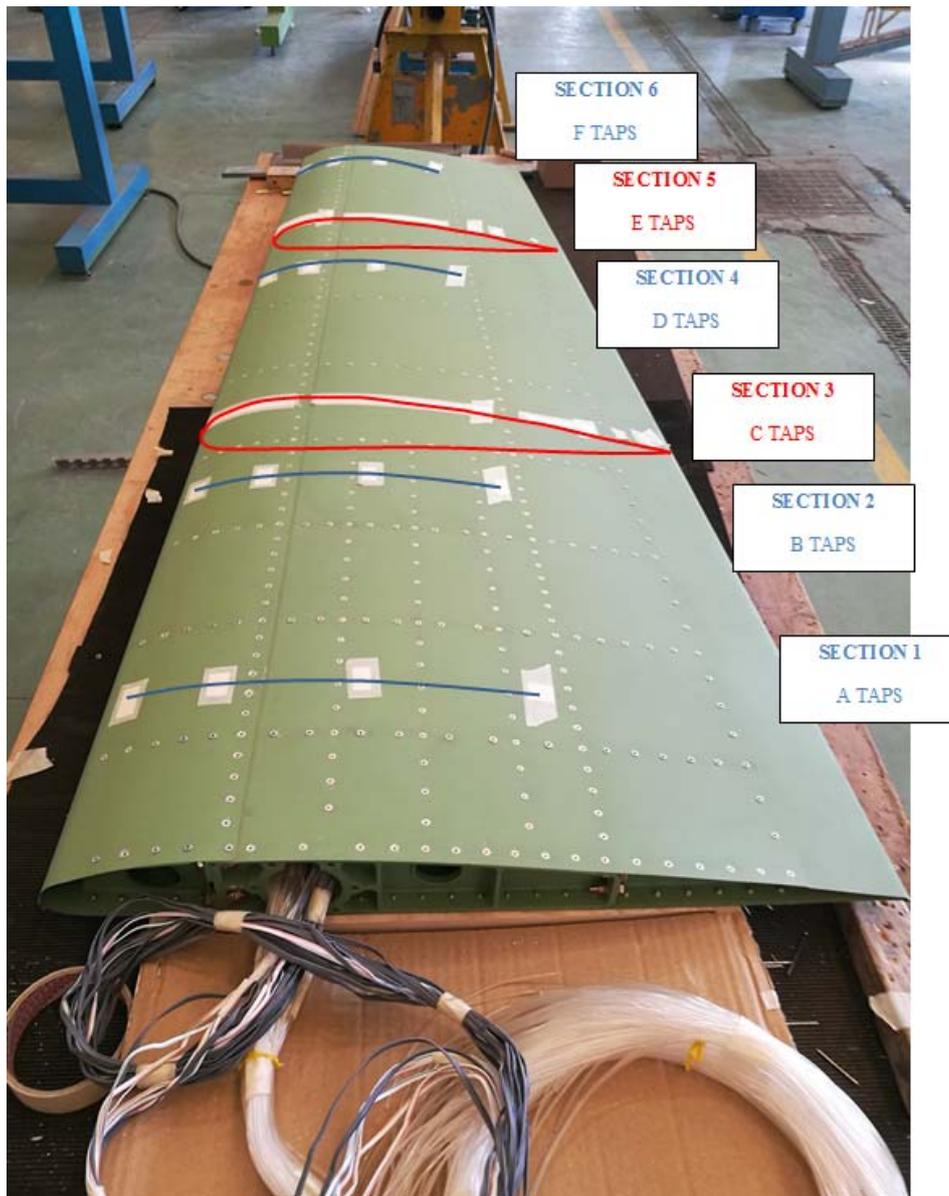
Figure 16 – Pressure taps on the final model.
