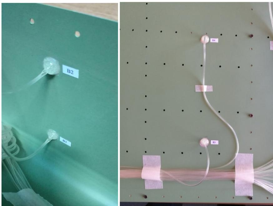
Figure 20 – Section B,  $y=450\text{mm}$ , pressure taps installed
