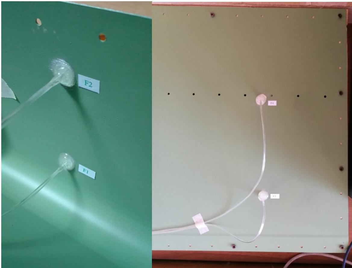
Figure 24 – Section F,  $y=1500\text{mm}$ , pressure taps installed
