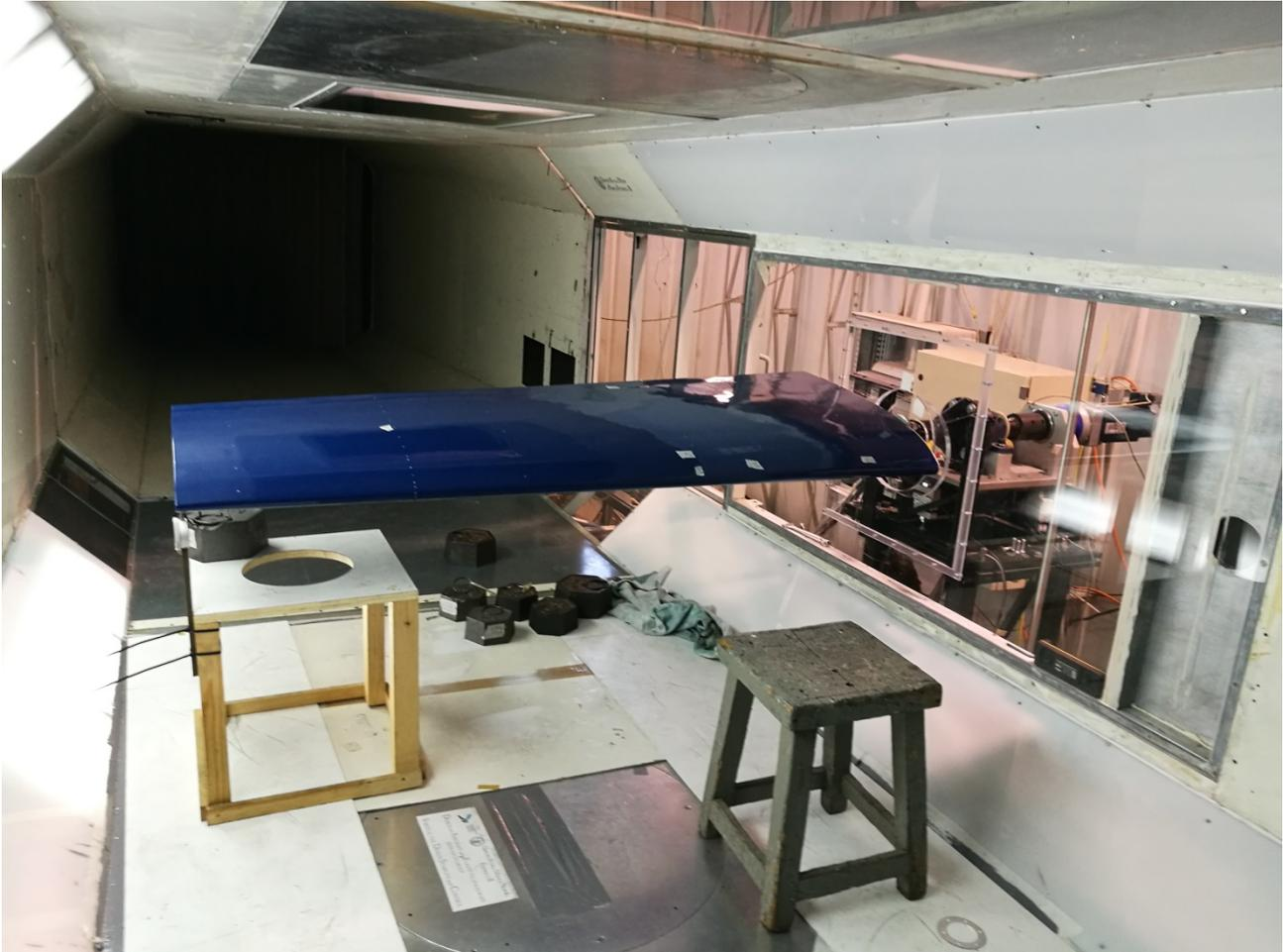
Figure 73 – Wing model in the UNINA wind tunnel facility.
