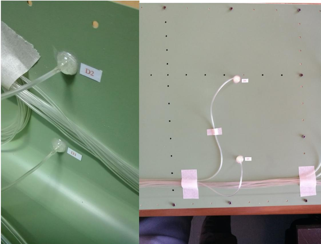
Figure 22 – Section D,  $y=990\text{mm}$ , pressure taps installed
