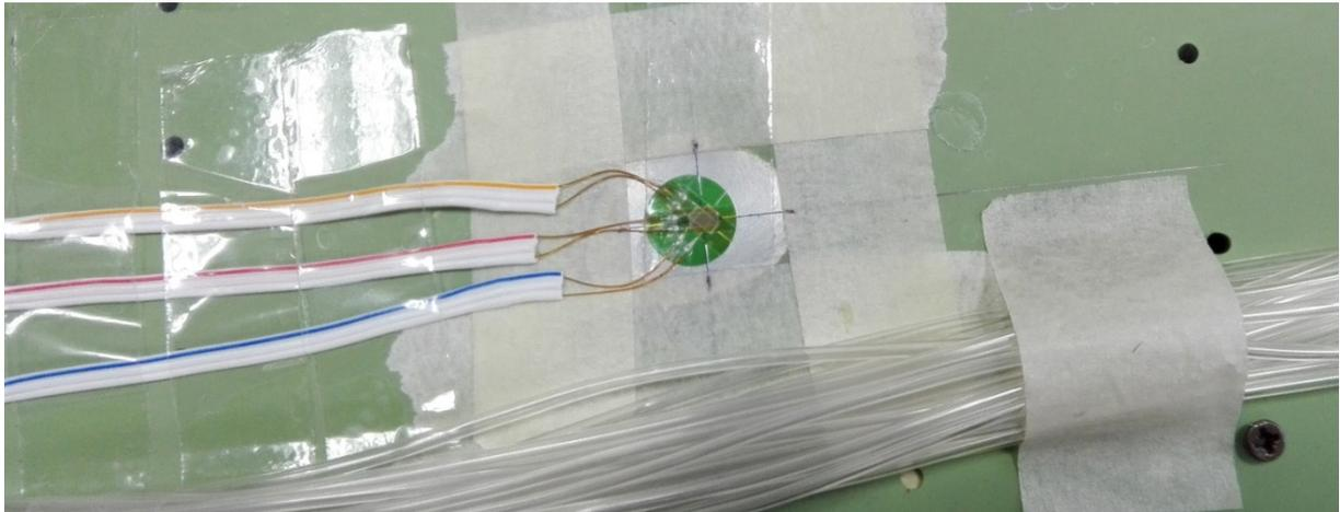
Figure 34 – Installation of SGs 18 on the upper skin.
