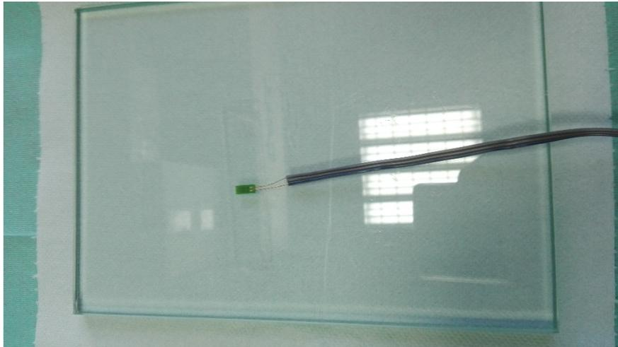
Figure 31 – Support surface for the preparation of SG before installation.
