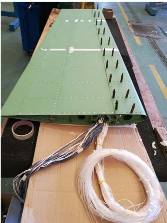
**Figure 67 – Leading edge positioning, bottom view**
