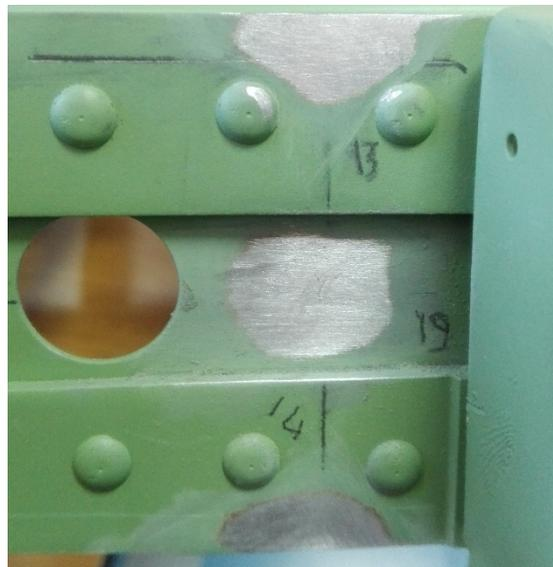
Figure 32 – Sanding of the aluminum surface around the location of SGs n. 13, 14 and 19
