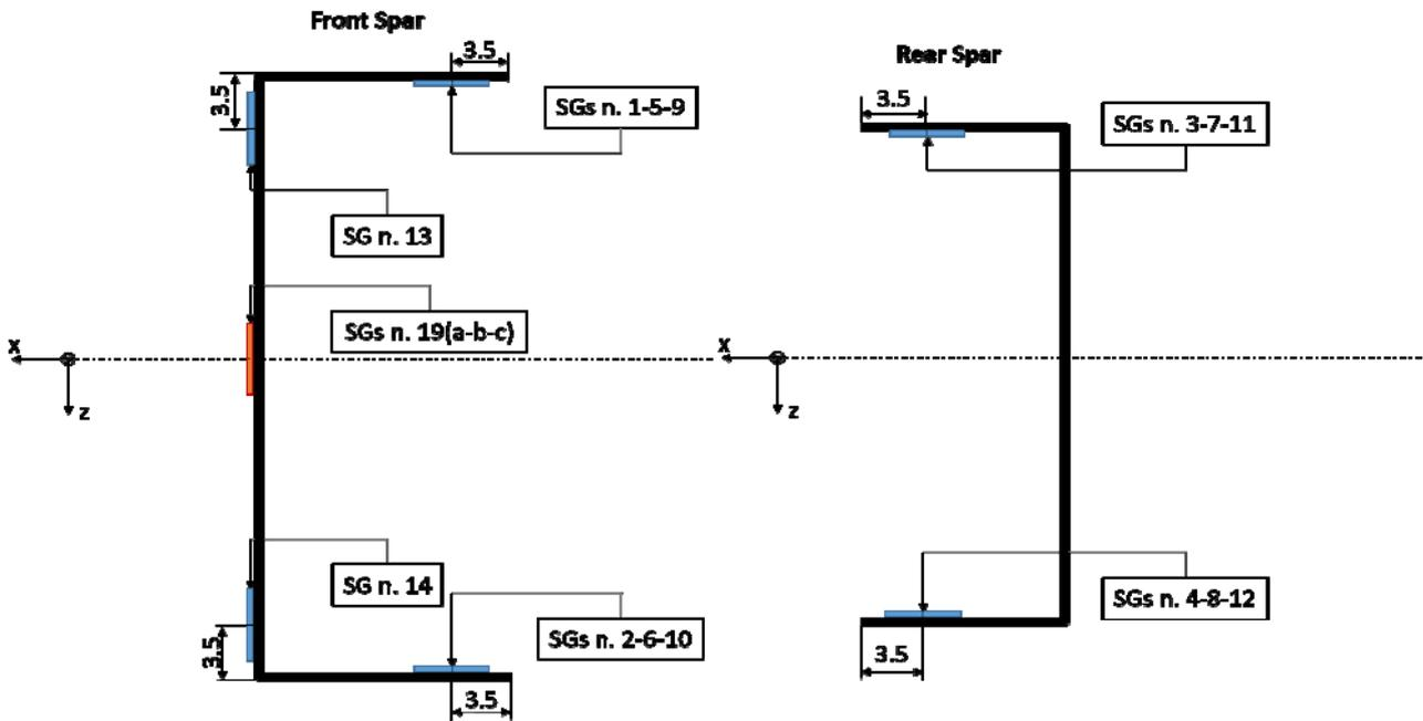
Figure 37 – Position of uniaxial SGs (blue elements) and rosette (orange element) installed on the spars. Distance reported are in [mm].
