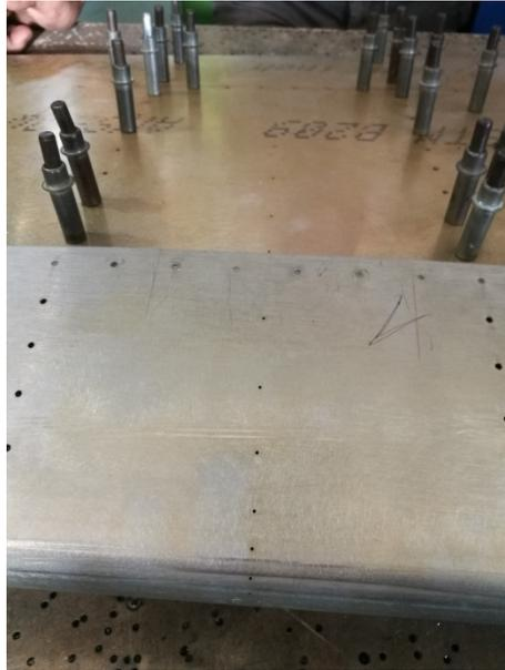
Figure 4: Alodine Treatment on the upper skin (details of pressure holes).
