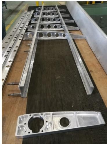
Figure 1: Detail of structural items during building, machined rib 1.
