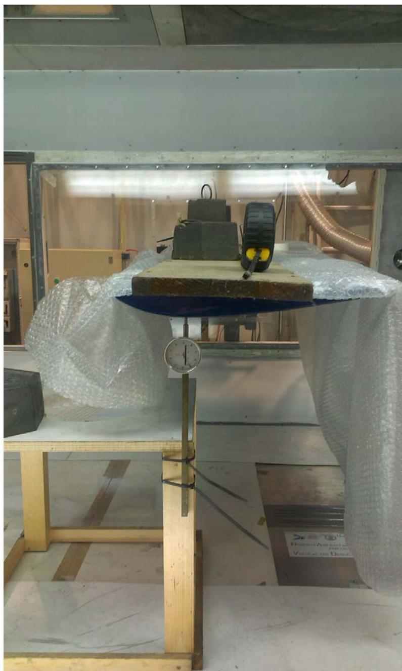
Figure 74 – Wing model in the UNINA wind tunnel facility, static loads test.
