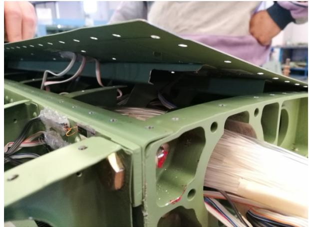
**Figure 62 – Upper skin positioning, detail of first stringer cutting**
