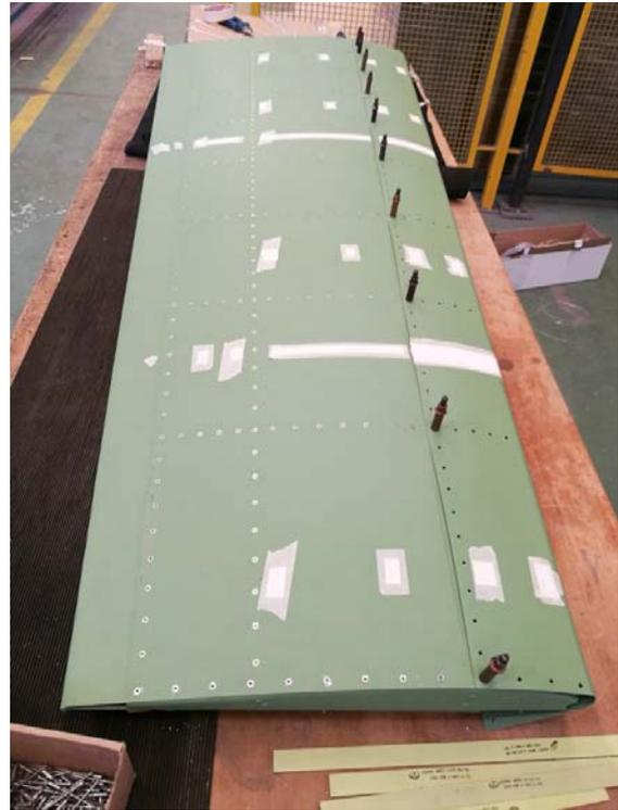
**Figure 66 – Leading edge skin positioning, top view**
