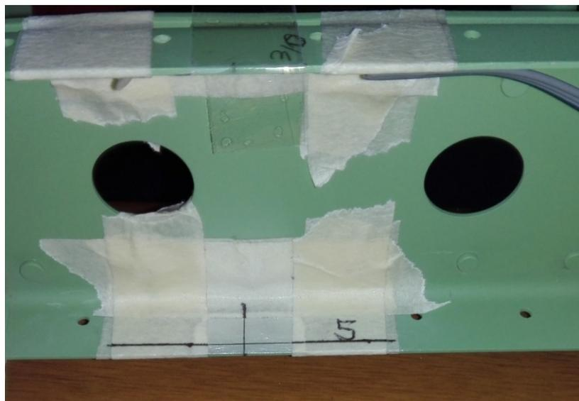
Figure 33 – Application of the masking around the delimited area sanded for the application of SG n. 5
