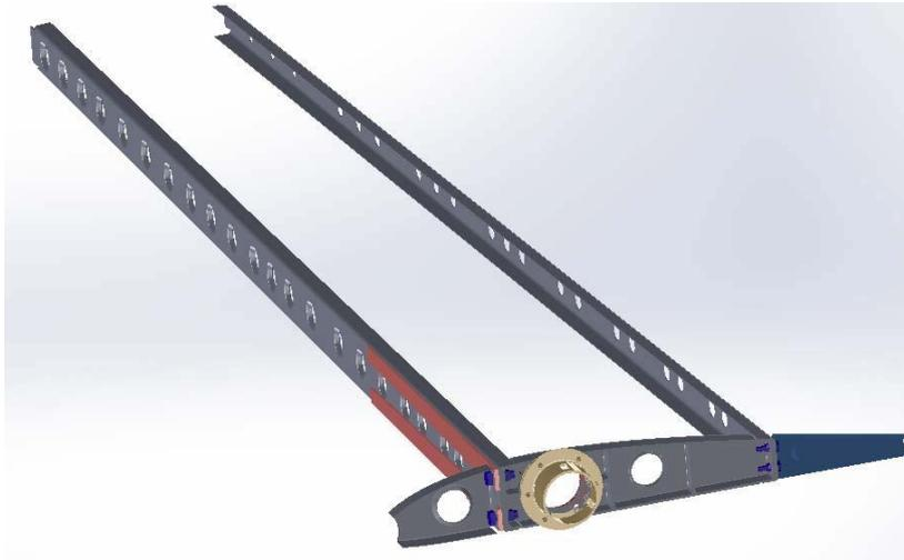
Figure 13: Spars and root rib
